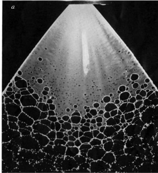
FIGURE 1. (Adapted from figure 28 in Dombrowski & Fraser 1954.) Perpendicular view of a planar sheet formed by injecting an emulsion of oil in water through a fan-spray nozzle. The oil droplets are heterogeneous nucleation sites, and sheet disintegration proceeds from the merging of holes. The image width is 5 cm; see also Rozhkov, Prunet-Foch & Vignes-Adler (2004) for a discrete impact of an emulsion drop on a solid.
