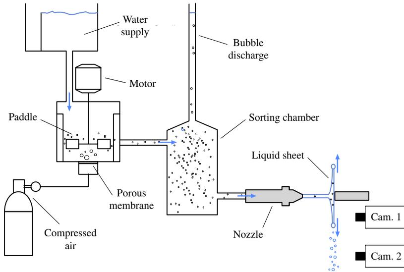
FIGURE 3. (Colour online) Experimental setup for the formation and observation of Savart water sheets seeded with small air bubbles.
