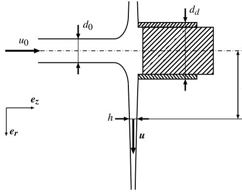
FIGURE 4. Detailed cross-section view of the jet impact. Note the jacket surrounding the solid cylinder, whose axial offset is adjusted in order to ensure a streamline deflection angle of  $\pi/2$ , to obtain a planar Savart sheet.
